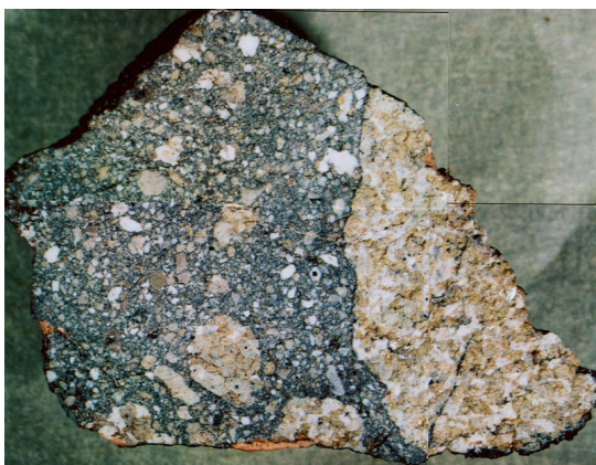
Figure 1a, b. NWA 2700 breccia and gabbro; slice (above) is 23 mm across, and cross-polarized thin section image of gabbro (below) is 7 mm wide.
