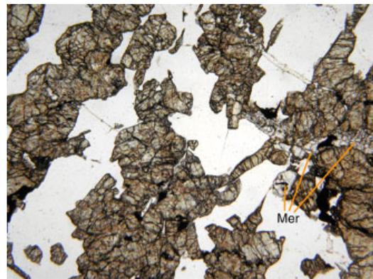
**Figure 3.** Plane-polarized (above) and cross-polarized (below, 2.35 mm wide) thin section images, showing pyroxenes (brown/colors), maskelynite (white/black) and oxides/sulfides (black).
